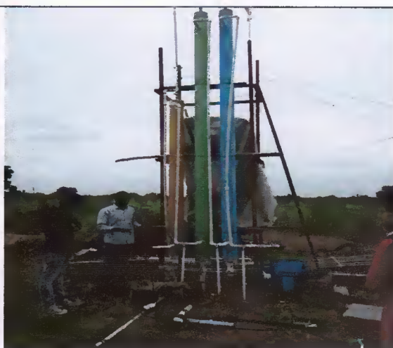
Field Visit of students to understand working of purification of generated Biogas
